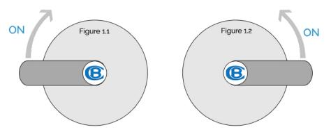
For wall lever taps we recommend this way for installing them as if the gland nut is loose (needing re-tensioning) gravity will push the tap to a close.
